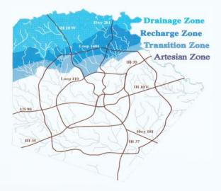
**The Drainage** or **Contributing Zone** catches rainfall and channels it down streambeds into the **Recharge Zone** where it enters the ground through caves, creek beds, faults, and fractures. The **Transition Zone** is less sensitive than the Recharge Zone, but is also vulnerable to contamination. Most of the water in the Aquifer is stored in the **Artesian Zone**.
